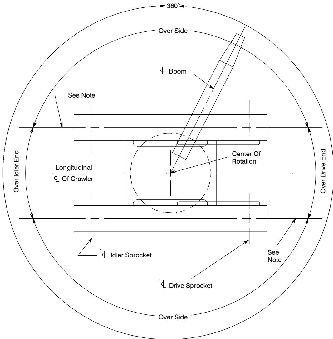
**Note:** These Lines Determine The Limiting Position Of Any Load For Operation Within Working Areas Indicated.
